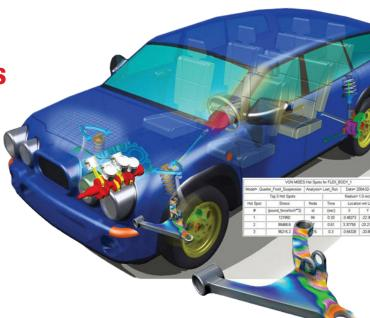
"Adams simulations permitted us to get different loading conditions to be studied through an FE analysis, putting to evidence the most critical loading combinations"
